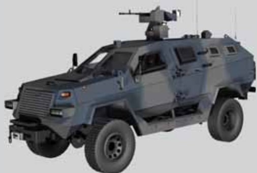
Remote Controlled Weapon Station with 12.7x108 mm NSV machinegun
