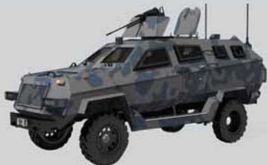
Open Turret with 12.7x108 mm NSV machinegun
